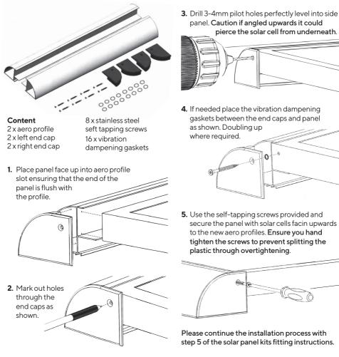
5. Use the self-tapping screws provided and secure the panel with solar cells facin upwards
