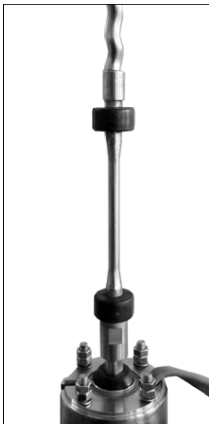
Figure 29: Motor with helical rotor attached, stator housing removed
